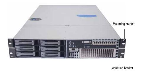
**2** Attach the handles to the sides of the server with two mounting screws on each side.
